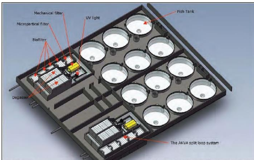
Figure 10. Scheme for FREA farm construction (Jokumsen & Svendsen, 2010, 37)
