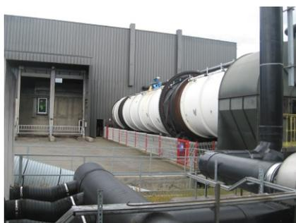
**mechanically separated part of mixed domestic refuse**. The process involves drying at 45° for 4 days, mechanical separation (sieving to 10mm, separation of heavy elements, of metals). Tests are also being carried out to compost green algae collected from Brittany's beaches.
