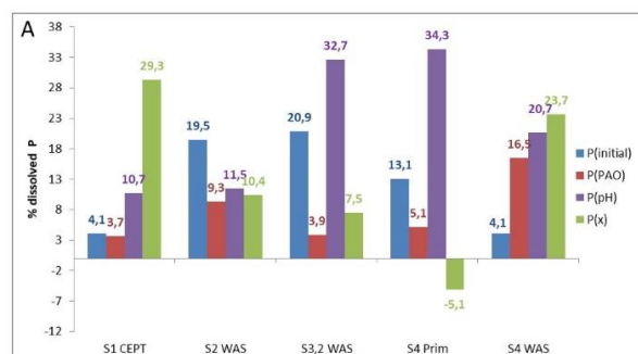
Figure2: Percentage of P dissolution by the different mechanisms induced by bioacidification. Sn: WWTP identification; CEPT: Chemically Enhanced Primary P removal; S2-WAS: EBPR+CPR activated sludge; S3-WAS: CPR activated sludge; S4-prim: primary sludge without Fe addition; S4-WAS: EBPR+CPR activated sludge; P(initial): P dissolved before BA; P(PAO): P released by the Phosphate Accumulating Organisms; P(pH): P released due to pH decrease; P(x): P released by other metabolisms (iron reduction)
