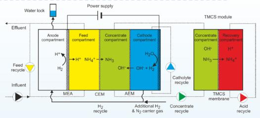
Fig 1. Scheme of the up-scaled electrochemical system for ammonia-nitrogen recovery. Source: P. Kuntke et. al, Journal ACS Sustainable Chemistry & Engineering (2018) 7638-7644.
