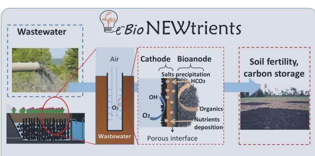
Fully-recyclable biochar-based METs modules, used in constructed wetlands for nutrients and carbon capture and recycling
