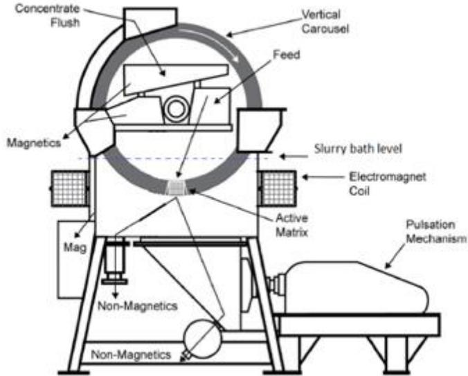
Vertical ring Pulsating High Gradient Magnetic Separator (VPHGMS)
