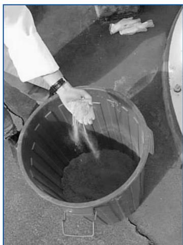
**Figure 1.** Photograph of MAP produced from the pilot-scale SC Process at the Oxley Creek wastewater treatment plant.
