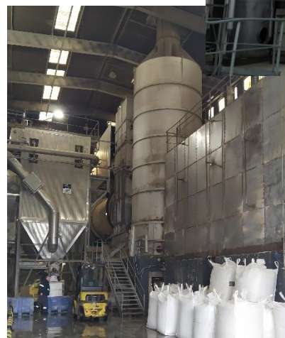
Cooperl site visit: digestate processing, organo-mineral fertiliser production from manure and animal by-products.
