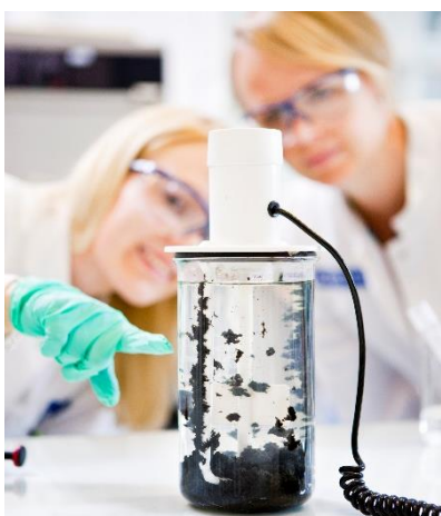
Photo: Regular verification of coagulant effectiveness in a wastewater sample (photo: Kemira).
